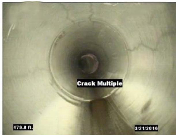
FIG. 7 Hinged Cracks (Multiple Longitudinal Cracks)
